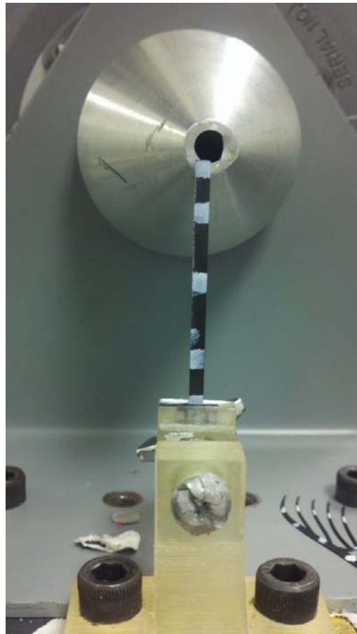
Figure 3.2: 40mm x 5 mm Beam with Airborne Excitation.
