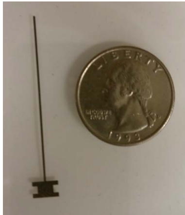
Figure 3.6: Test Specimen for Ply-Orientation Test.
